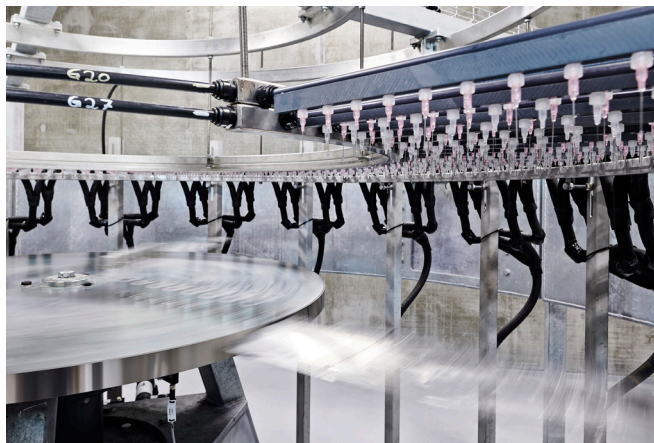
620 nozzles simulate realistic rainfall.
